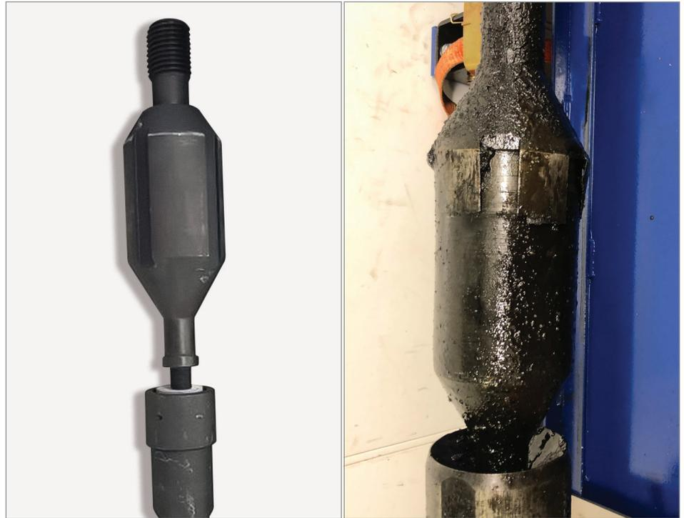
Centralizer (left) and milled centralizer recovered to surface (right).
