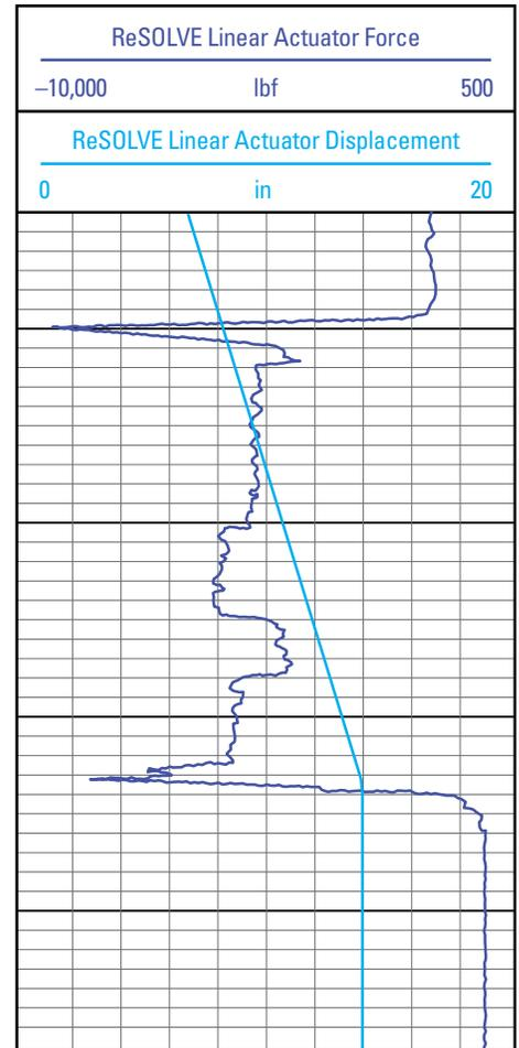
Successful shifting to open each of the 10 ICDs in the horizontal well is shown by the expected displacement and force signature that matches the reference log made at the surface.
