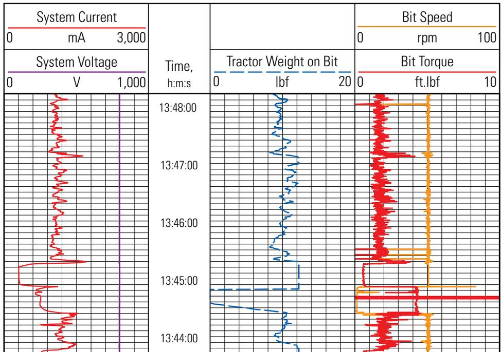
The ReSOLVE service's log documents the precision of the MillOptimizer system in automating a milling operation.
