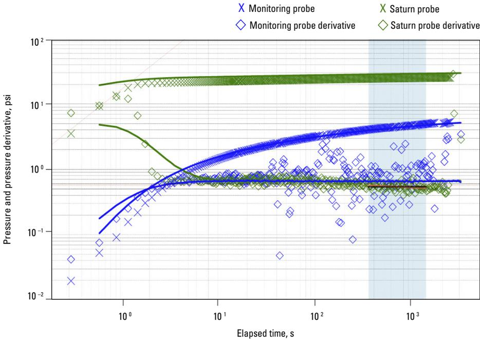
*The consistency of the superimposed radial flow regimes achieved by the pressure gauges in the Saturn 3D radial probe and the monitoring probe provides high confidence in the results. The derivative plot from the Saturn probe does not have a distinct spherical flow regime; permeability anisotropy is interpreted from simultaneous matching of the Saturn and monitoring probe pressures.*
