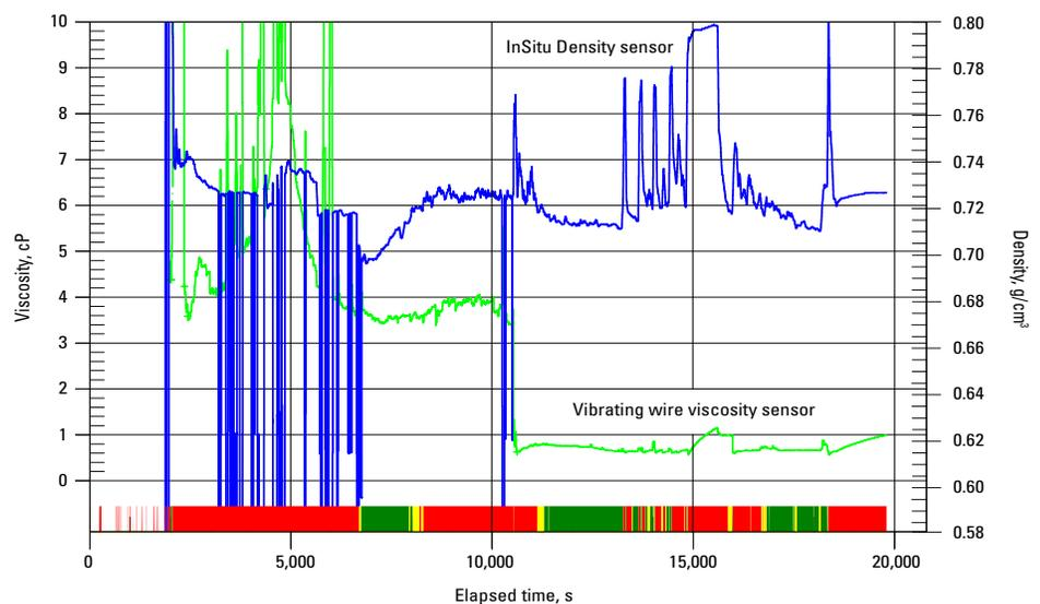
High-quality measurements (flagged green in the bottom track) of density by the InSitu Density\* fluid density sensor and viscosity by a vibrating wire sensor were made on fluid flowed from the higher mobility upper zone.
