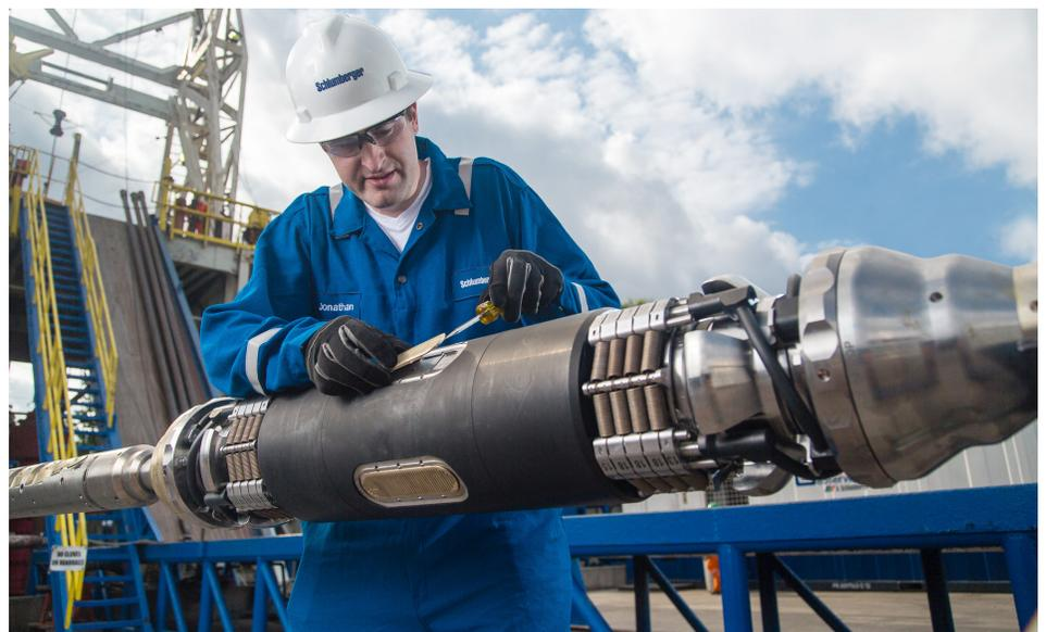
The compact drain assembly of the Saturn 3D radial probe reliably seals to the borehole to directly flow fluid from the formation.
