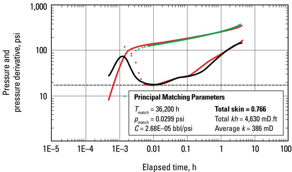
Analysis of the drillstem test conducted after perforating indicated a total skin of only 0.766, which is a more than 60% reduction from the skin estimated for conventional perforating. T = time, p = pressure, C = wellbore storage constant, k = permeability, h = height.
