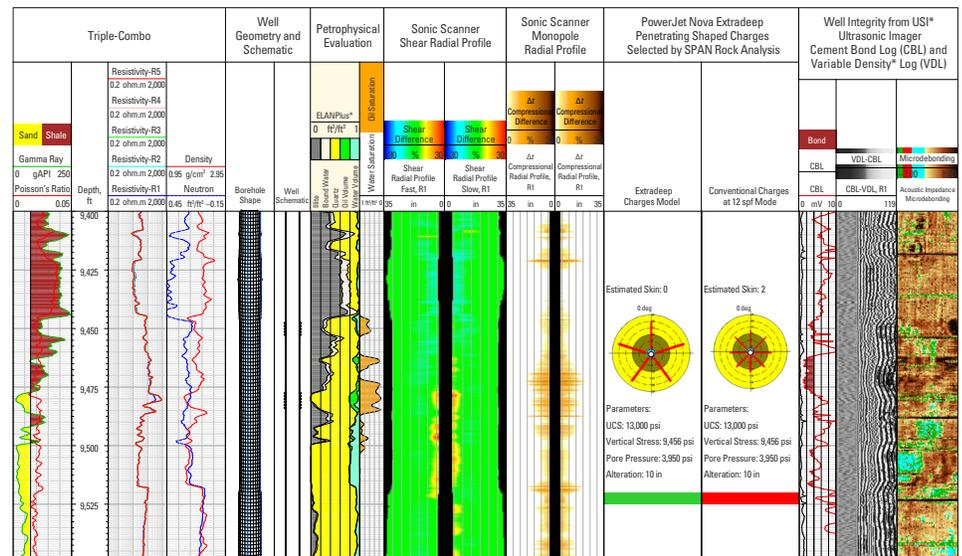
SPAN Rock analysis incorporated high-quality acoustic measurements by the Sonic Scanner platform to fully account for the depth of alteration and geomechanics of the formation. The recommended PowerJet Nova extradeep penetrating charges successfully penetrated beyond the alteration zone.
