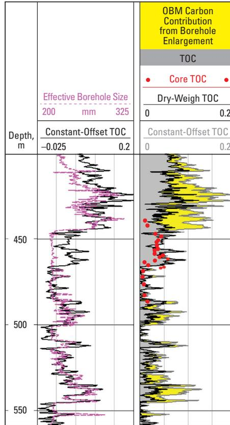
The conventional constant carbon offset does not track well with the varying borehole size in the left-hand track. In the right-hand track, the good agreement of TOC measurements on core plugs (red dots) with TOC obtained using the borehole correction methodology with Litho Scanner service's measurements (gray shading) verifies the accuracy of the correction. The yellow shading shows the magnitude of the correction for OBM carbon from borehole enlargement.
