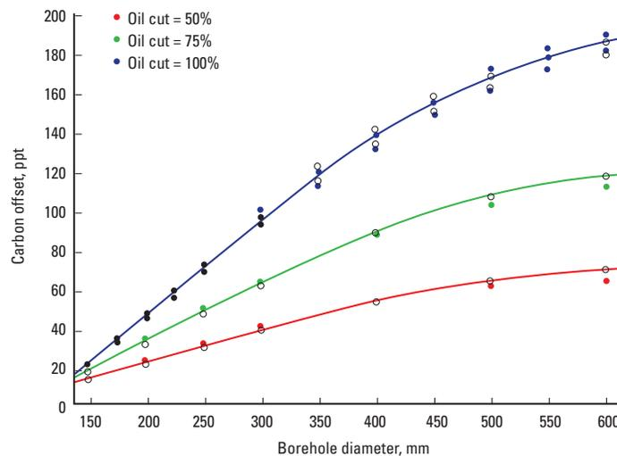
Modeling was used to calculate the carbon offset correction as a function of borehole size and OBM oil/water ratio.
