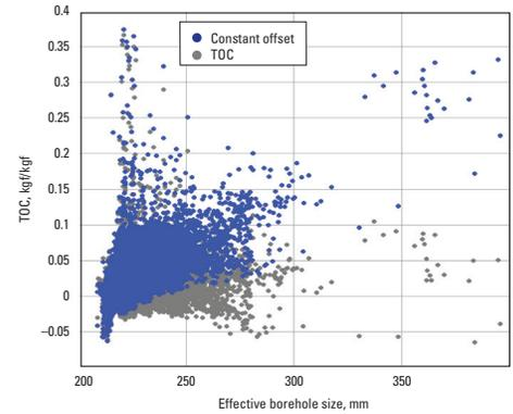
The borehole-corrected TOC (gray) does not correlate with borehole enlargement, but the constant-offset TOC (blue) does because it fails to account for the variation of the OBM carbon signal with hole size and shape.
