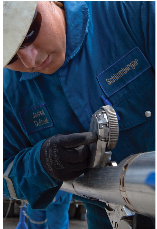
The bidirectional, high-speed TuffTRAC tractor uses traction control to continuously monitor and adjust the radial force applied by the tractor arms.
