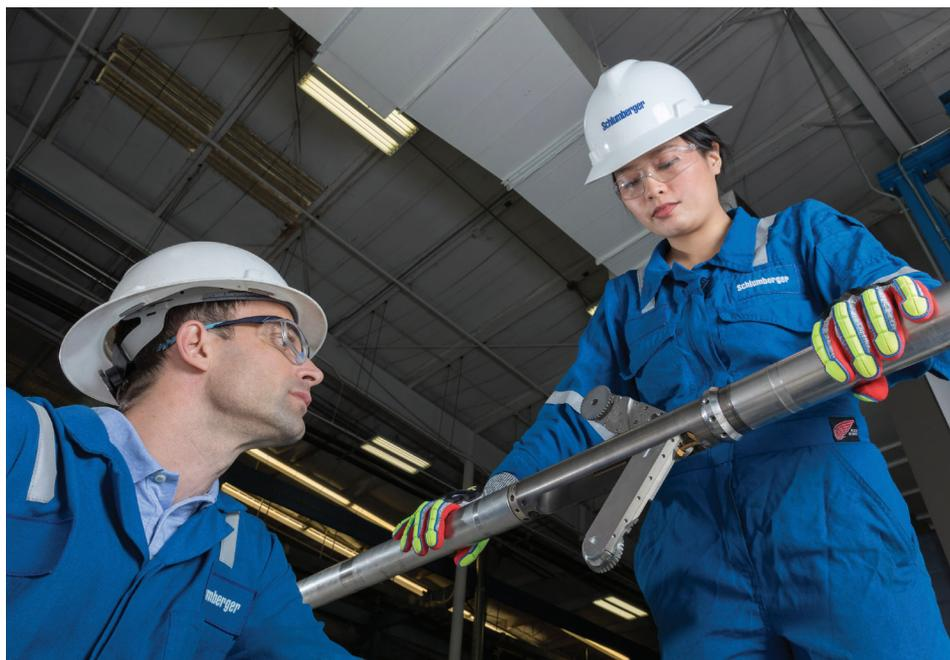
*The compact TuffTRAC iX tractor's four drives are operated independently for unprecedented maneuverability and optimized low power consumption.*
