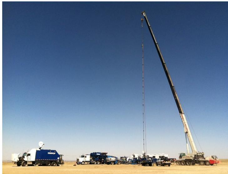
*By deploying ReSOLVE intervention service on the versatile, high-force UltraTRAC tractor, only a 130-ton crane and logging unit were needed to conduct the successful fishing job.*
