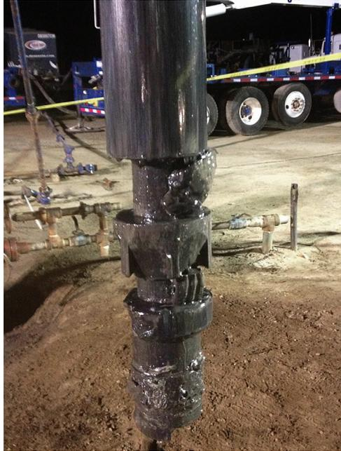
*The partially set bridge plug could not be freed and recovered using a conventional tractor without exceeding the cable's maximum safe pull.*
