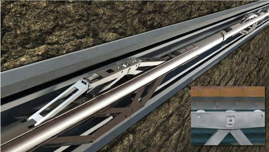
*The MaxTRAC tractor uses an inchworm traction system based on two or more tractor sections. As one section grips the casing or formation, the next is resetting for continuous motion.*
