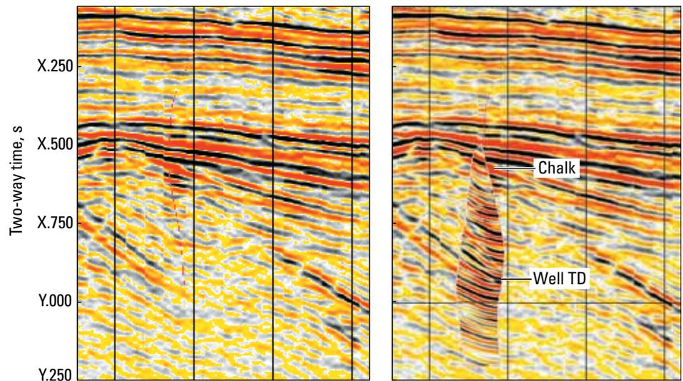
*Because the surface seismic image was produced using chalk velocities that are too low (left), it fails to tie with the VSP (small region with higher amplitudes and higher resolution, narrowing upward on the right). The mismatch is obvious in several intervals.*
