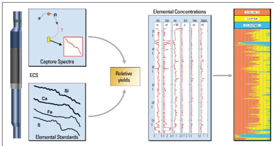
*It was possible to accurately estimate elemental concentrations using SpectroLith lithology processing of spectra from neutron-induced gamma ray spectroscopy tools to process the ECS data.*
