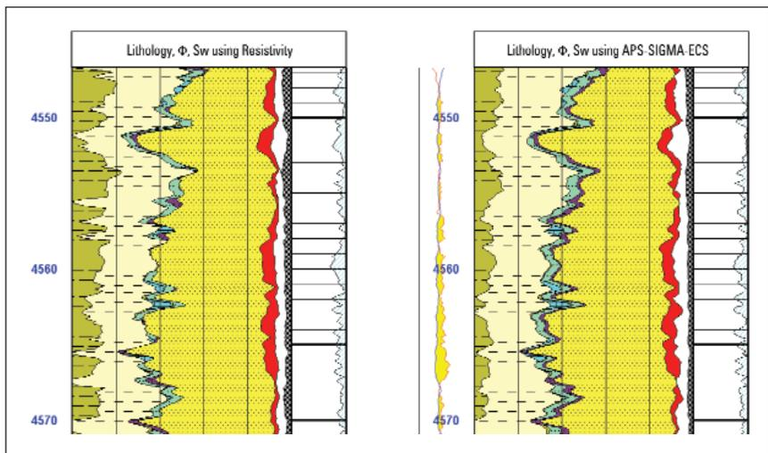
*Comparison of two petrophysical evaluations over the same section provide data with resistivity (left) and without resistivity using the APS-Sigma-ECS method (right).*
