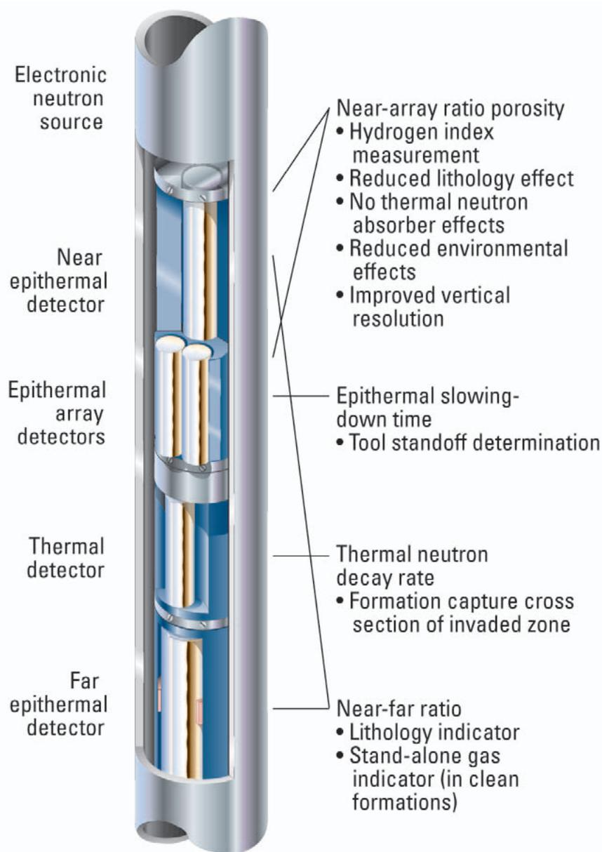
Neutron detectors in the APS tool are positioned eccentrically, borehole-shielded, and focused toward the formation.
