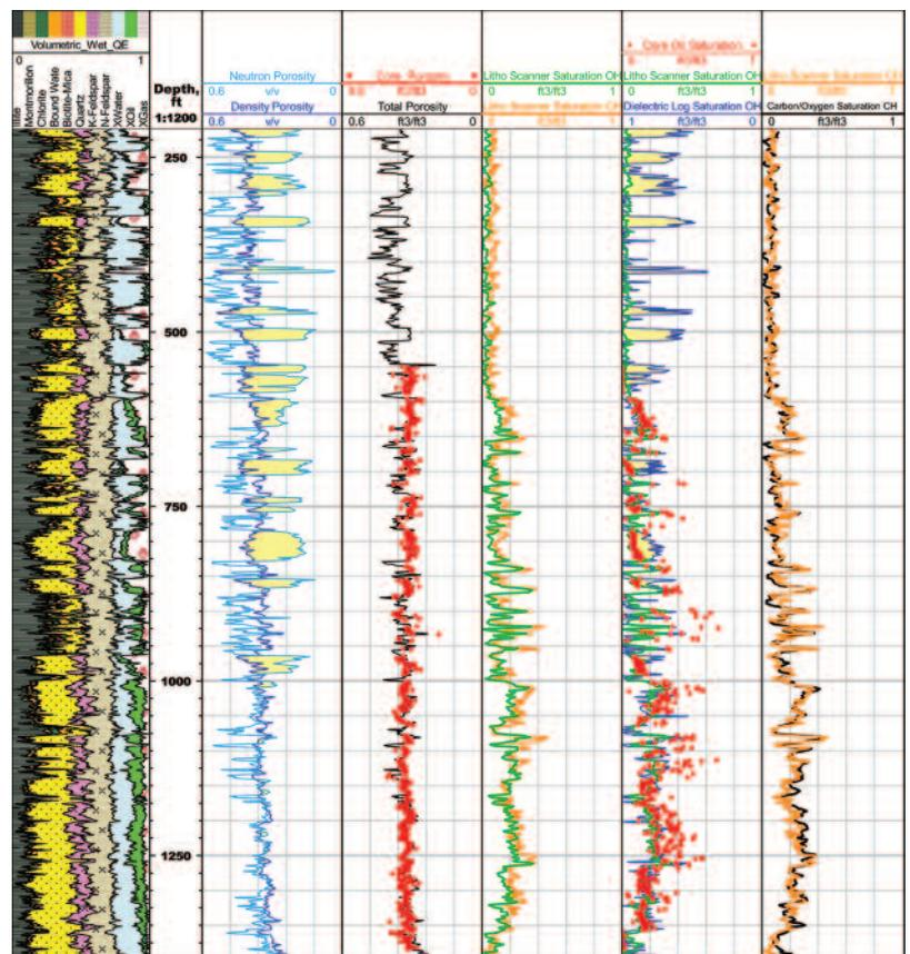
**FIGURE 2. Hydrocarbon saturation is difficult to determine with conventional approaches due to residual effects of EOR involving steam injection. However, saturation determined from the Litho Scanner service in both open- and cased-hole conditions yields accurate results, as confirmed by core and other log measurements.**
