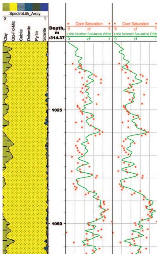
**FIGURE 1.** Hydrocarbon saturation based on TOC as determined by the HD spectroscopy service logging in both water- and oil-based mud in a complex formation in Canada closely matches core measurements. (Images courtesy of Schlumberger)
