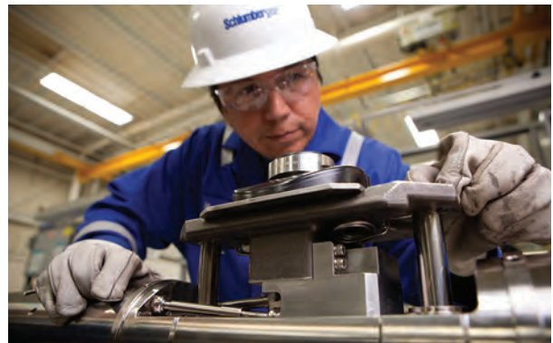
The MDT wireline formation tester makes real-time flowline resistivity measurements at the probe module to discriminate between formation fluids and filtrate from water- and oil-based muds. (Courtesy of Schlumberger)
