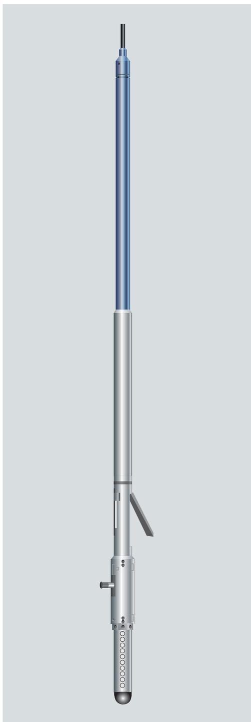
The standard configuration of the rotary Mechanical Sidewall Coring Tool (MSCT) recovers 50 core samples. Optional configurations for recovering 75 core or 20 core-catcher (dictated by core-catcher capacity) samples are available. Each sample is isolated for positive identification, and a summary output at surface lists all samples with the exact depth and time that each was taken.
