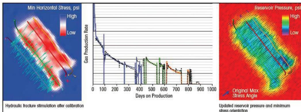
**FIGURE 2. The second phase of the modeling process focused on assessing how depletion changed the in situ stress magnitude and orientation. (Source: Schlumberger)**
