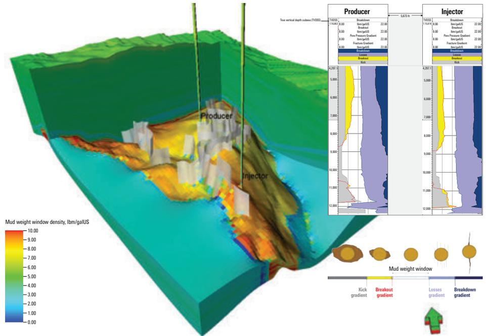
The 3D geomechanics model generated using Petrel Geomechanics and VISAGE simulator enabled Ithaca Energy to optimize its completion design, investigating possible occurrence of sanding and screening water-weakening effects during injection.
