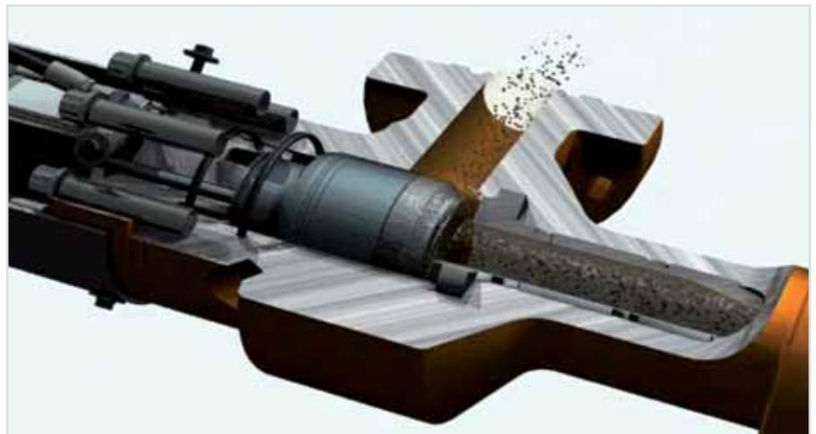
Cut-away of the AutoChoke system in operation
