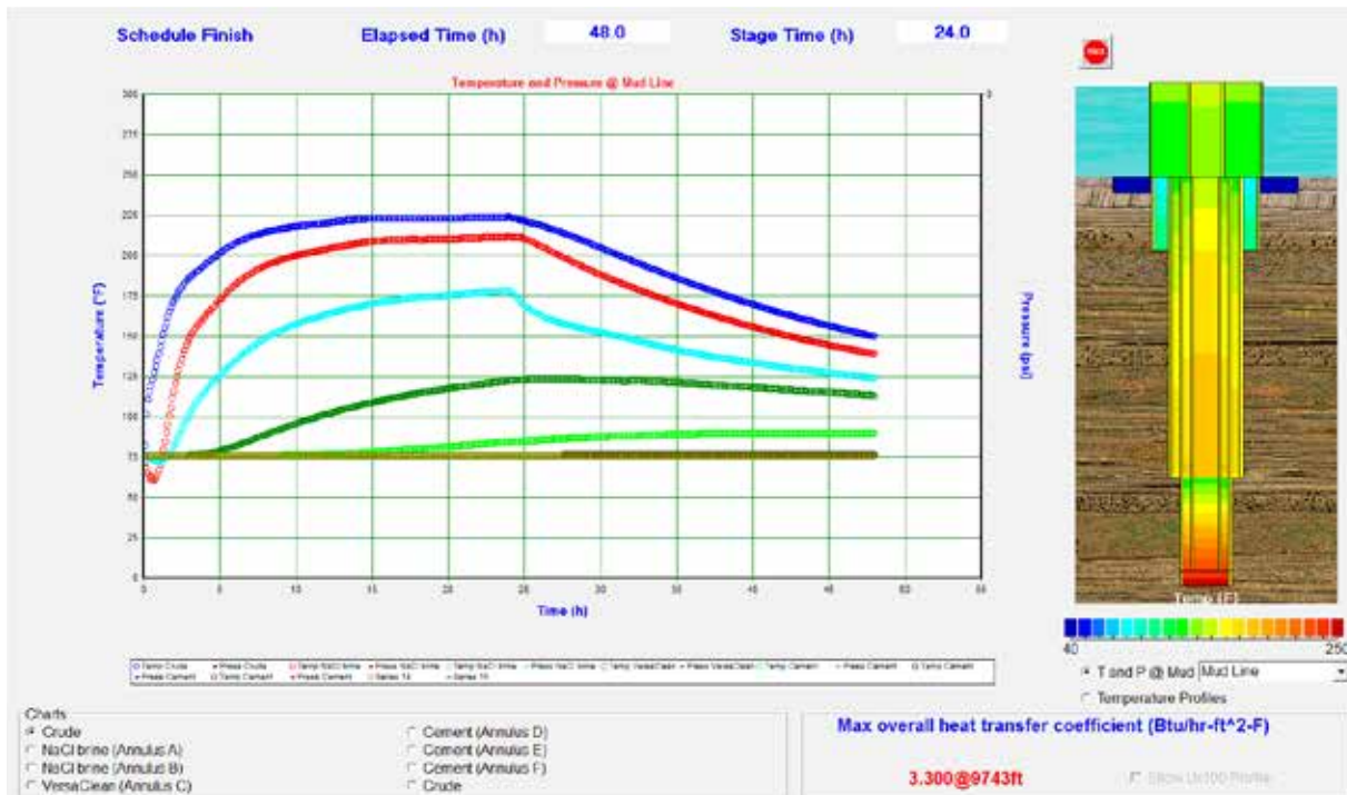
Production and shut-in with brine in annulus. Final crude temp 150 degF (66 degC).
