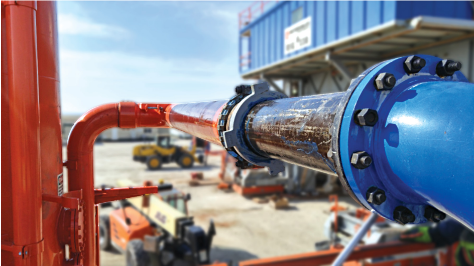
The hydraulically deployed U-tube enables a quick connection to the rig flowline.
