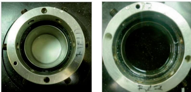
Figure 1- Competitor's Initial 4 hour filtercake (left) and residual filtercake (right) after 72 hr soak
