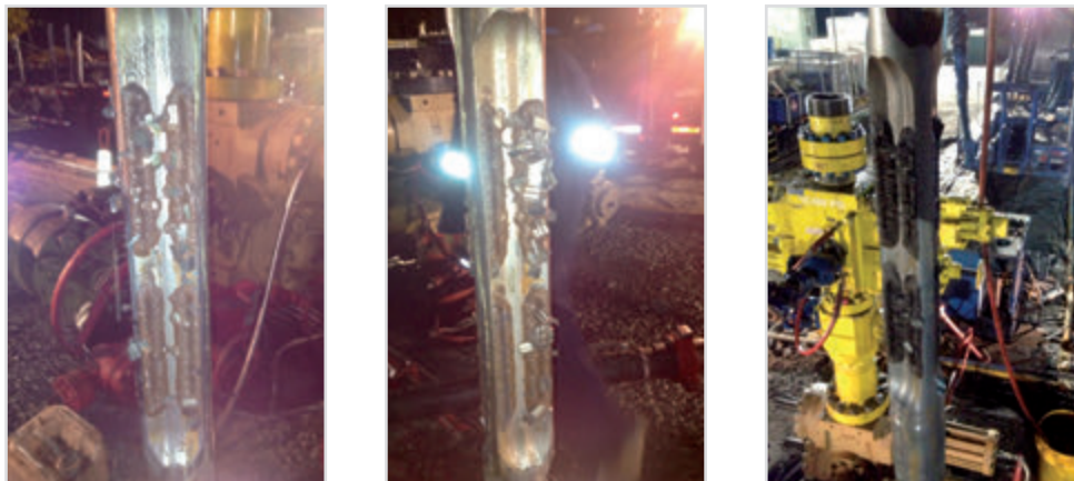
Pictures of the three sides of the CT MAGNOSTAR magnet as it was retrieved at surface after the milling operation.
