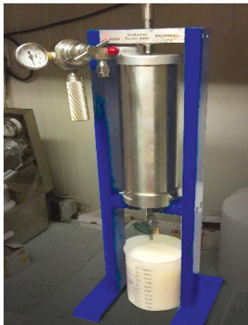
*The production screen test, provided by M-I SWACO, demonstrated that the solids-free DIPRO LD fluid chosen for this well would not clog screens.*
