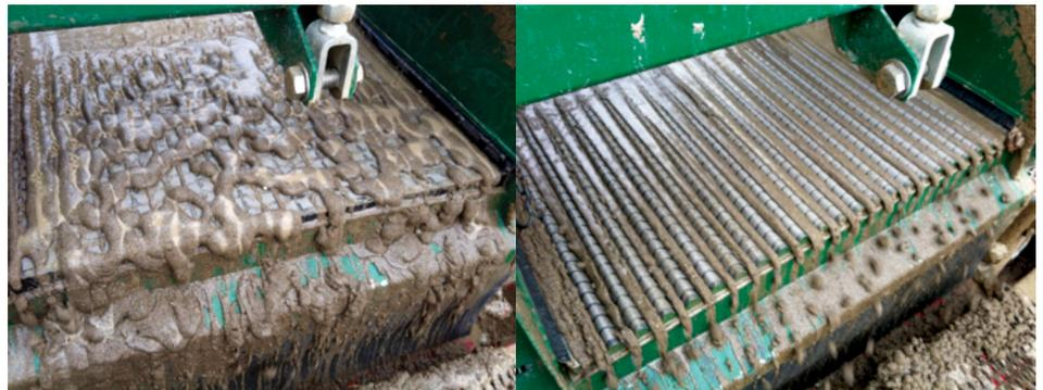
*The DURAFLO D500-C replacement screen maintained even flow distribution across the entire screen (left). In contrast, the OEM corrugated-hook-strip panel generated solids-induced valleys and inefficient use of screen area (right).*
