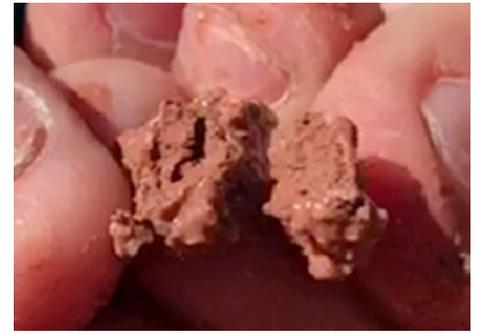
*Dry cuttings from the primary shakers demonstrate the inhibitive properties of the HydraGlyde fluid system.*
