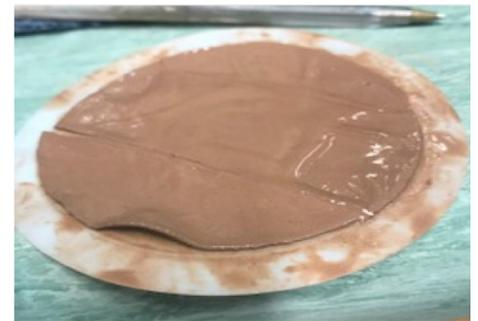
*The HydraGlyde fluid system deposits a thin and flexible filtercake.*
