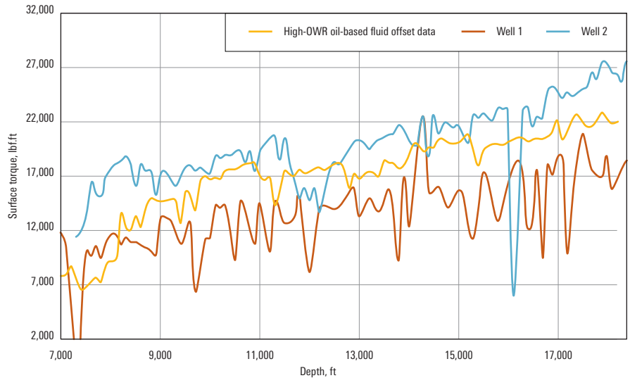
An offset well with a high-oil/water ratio fluid was compared with the surface torque of the HydraGlyde system wells in the same area. HydraSpeed lubricant was added halfway through the first well at 1% volume. The second well maintained a HydraSpeed lubricant concentration of around 1 to 2% volume.
