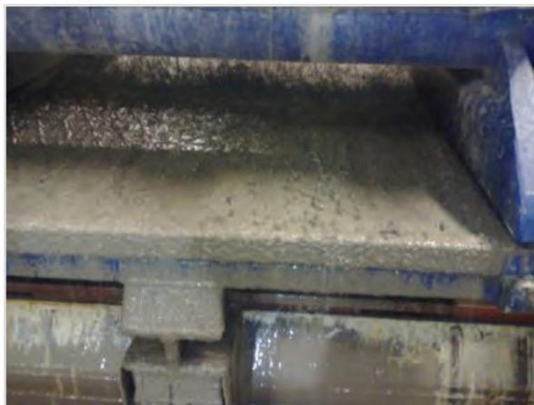
Cuttings on shale shaker while directional drilling
