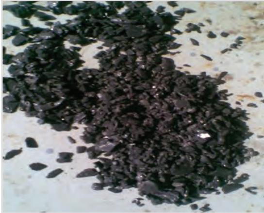
Cuttings on shale shaker while directional drilling
