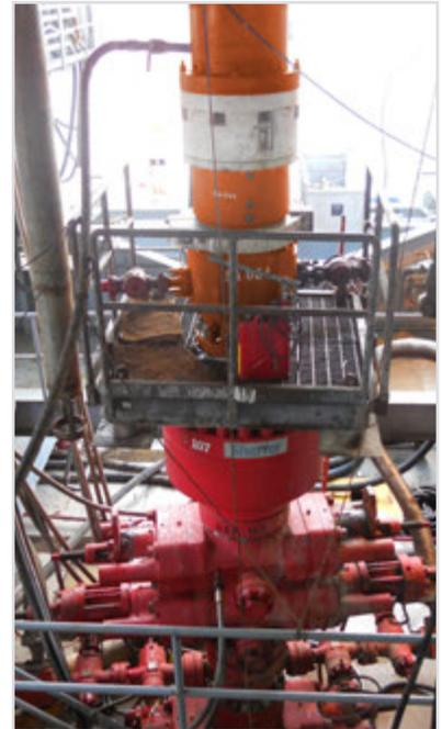
Figure 5: HOLD RCD on top of annular preventer
