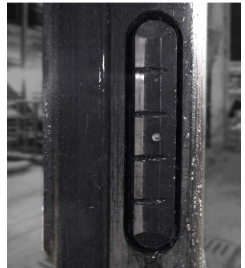
SWITCHBACK SCRAPER tool scraper blades in the recessed position.
