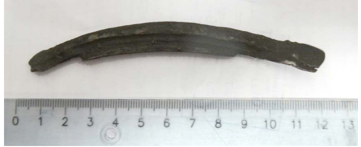
A large piece of ferrous debris recovered by the SWITCHBACK SCRAPER tool and MAGNOSTAR magnets.
