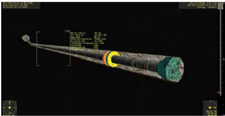
VIRTUAL HYDRAULICS helps maximize drilling fluid performance and minimize drilling costs. The pressure analysis generated by the software was used to mitigate risk of soil failure as a result of hydro-fracture and maintain stability of the borehole.
