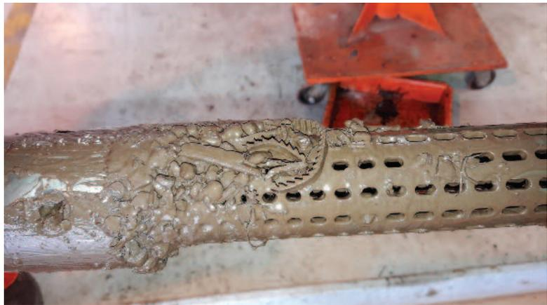
**The same 4¾-inch work string filter was run consecutively in seven extended-reach shale wells in Argentina, capturing more than 10 pounds of fluid-borne circulation debris with no replacement screens.**
