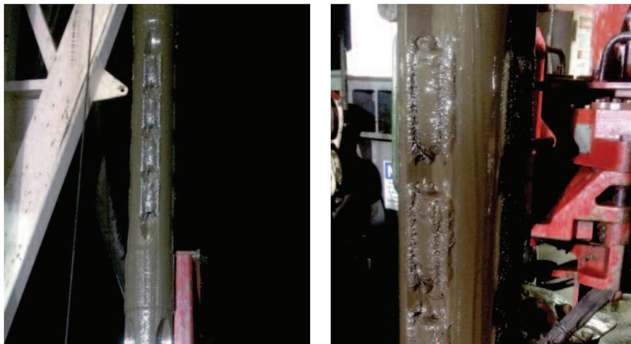
In an extended-reach horizontal drilling campaign in the Permian Basin's Wolf-bone play, the open-hole magnet removed 33 pounds of ferrous debris while drilling. After installing the magnet, the company drilled the horizontal 8½-inch section to nearly 30,000 feet TD with no steering issues or formation damage.
