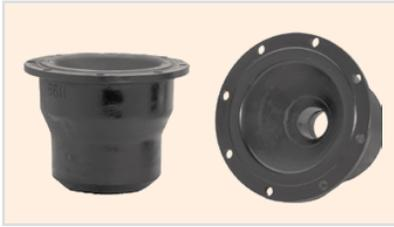
Standard sealing element, secured to drive bushing with cap screws and locking wire, can strip tools up to 8¼-in OD.
