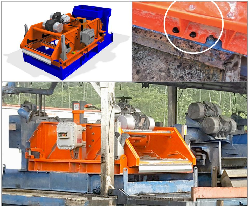
*The MONGOOSE PRO shaker retrofit kit enables easy replacement of worn, damaged, or poorly functioning shakers quickly with an easy no-weld, bolt-on installation.*
