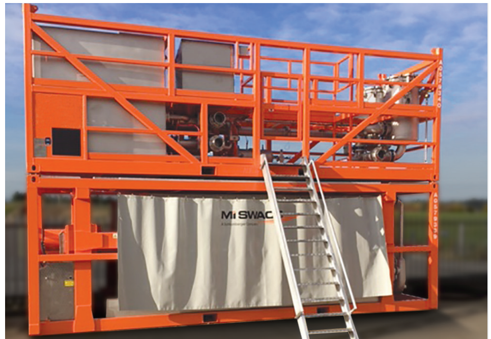
The Torrential high-flow filtration unit is capable of handling high-processing rates exceeding 15 bbl/min [2.39 m 3 /min].
