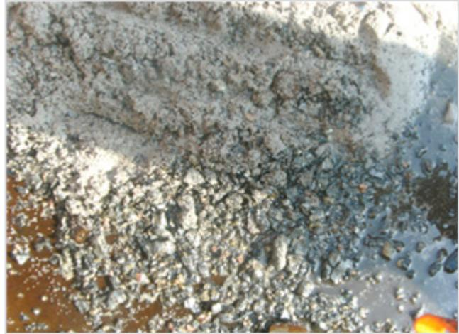
Non Ferrous Debris Recovered in Debris Chambers
