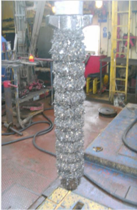
Ferrous Debris Recovered in Debris Screening Module
