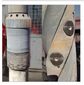
M-I SWACO developed the WELL DOMINATOR sub tool to extend the capabilities of the WELL COMMISSIONER tool. By using the same packer for both tests, the operator was able to drill cement and test the well in a single run—completing the job in record time for monobore wells and saving 2.5 days.
