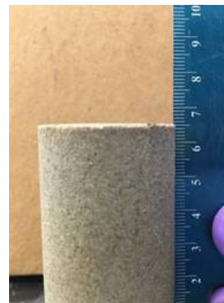
Core plug after breaker soak and flowback showing complete removal of the filtercake.
