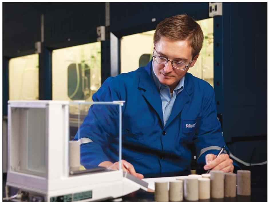
^ Weighing core plugs. Precision weighing of every sample at each stage in the cleaning and extraction process is required because small differences in weight affect grain density calculations and subsequent determination of other important reservoir parameters such as fluid saturation.
