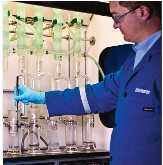
^ Dean-Stark apparatus. A core analyst inserts a core plug into the sample chamber (photograph). The typical setup (left) consists of an electric heating element, or heating mantle, a boiling flask with extractor chamber, a sample thimble or support screen, a water trap or calibrated receiving tube, and a condenser. The Dean-Stark method results in a quantitative measure of water volume extracted from a core, and therefore each sample is cleaned individually in a separate apparatus.
