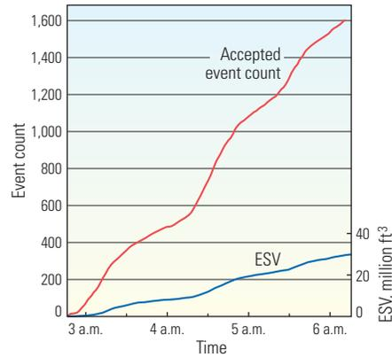
◀ Effective stimulated volume. Analysis of the event cloud density provides a measure of the effective stimulated volume (ESV) of rock within the formation (*left*). The irregular surface excludes outlying events. This analysis provides a real-time diagnostic tool (*above*). An increase in the cumulative number of events (red) with a simultaneous increase in ESV (blue) indicates growth in the volume of the fractured-rock zone.
