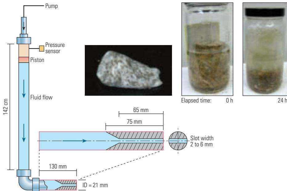
^ Diversion testing. The laboratory setup for testing fibers in proppant slurries used a long tube with a removable, adjustable slot (diagram). After each test, the slot was disassembled and a visual check of the fiber and proppant bridge that formed in the slot (photo, left) confirmed the pressure increase seen during the test. Photos of the laboratory vials show degradation of the plug begins within one day.
