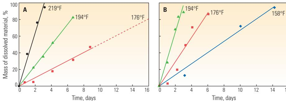
^ Fiber degradation in the presence of additives A and B. Over time, the polyester comprising the fibers degrades into shorter-chain polymers, eventually leaving only a safe, water-soluble weak acid.
