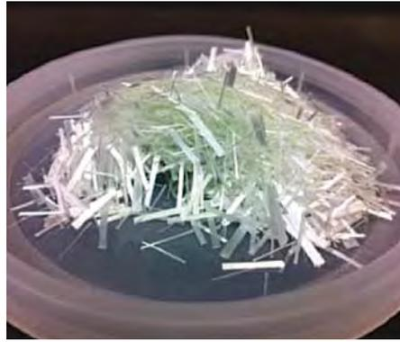
▲ PressureNET treatment. PressureNET technology combines the strength and light weight of a lost circulation material such as vitrified shale particles (*left*) with the strength of CemNET fibers (*right*).
