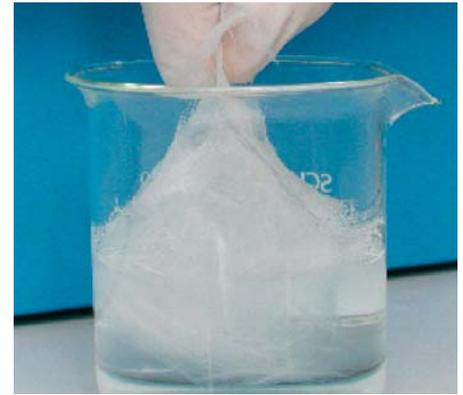
^ CemNET engineered fiber technology. Dry CemNET fibers (left) form a sheet-like network when mixed with water (right), enabling the network to seal lost circulation zones. CemNET fibers are dispersible in any cement system and can be added and mixed quickly in a mixing tank.
