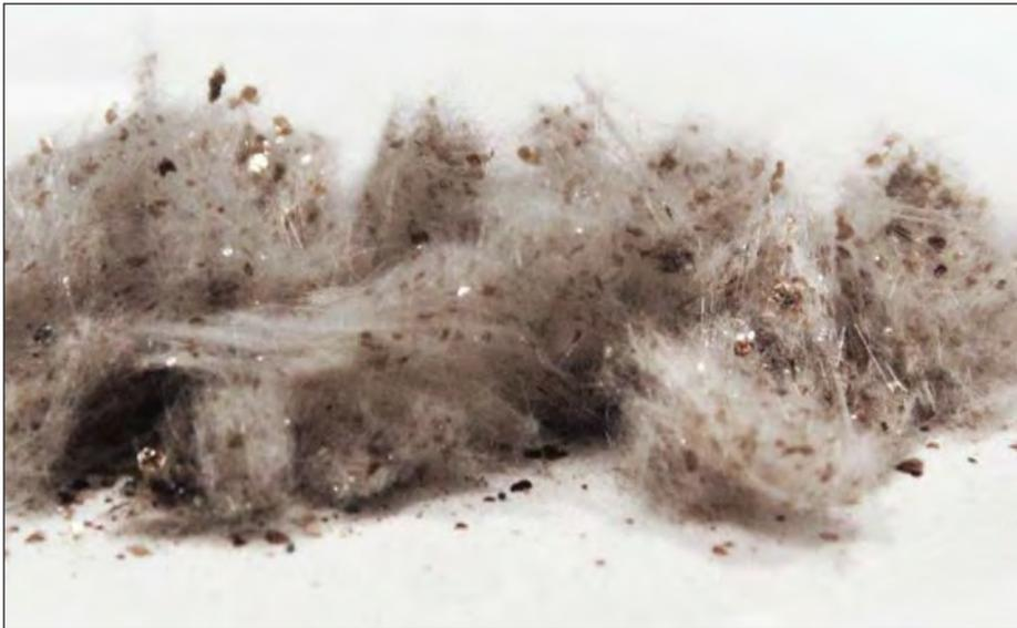
^ Losseal microfracture material. The Losseal microfracture solution is an engineered fiber treatment, combining specific fibers (light gray) with solid bridging materials (dark gray).
