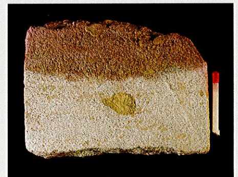
□ Laminated shale clast, Frio sandstone, South Texas. This clast, a little larger than an electrode of the Formation MicroScanner tool, would appear on the image as black against a light background. The overlying clay-rich bed would appear a darker gray than the sand.
