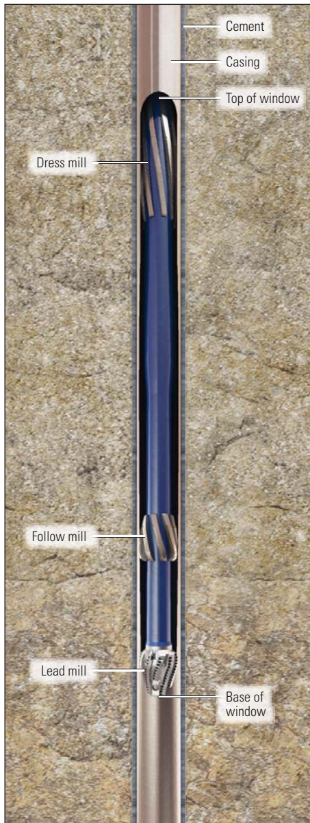
^ Milling a window. The TrackMaster CH whipstock system uses specially designed mills to create a window exit through the casing. After the last mill has passed through the casing, the mills are typically pulled, and a directional drilling assembly is run to total depth.
