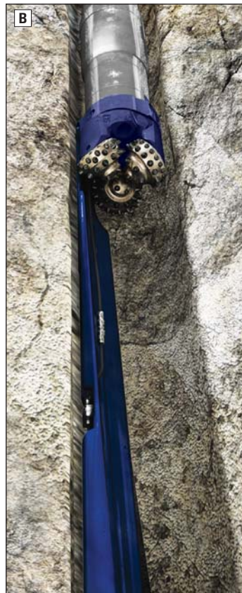
^ Bit and mill options. The bit or mill is attached to the top of the whipstock before it is run in the hole. On an openhole assembly, the bit is attached to the whipstock by shear pins. The openhole system can accommodate PDC (A), roller cone (B) or diamond-impregnated bits (C). Cased hole mills (D) are attached to the top of the whipstock by a break bolt. After the whipstock is oriented and the anchor is set, the bit or mill is separated from the whipstock by exerting upward or downward force to shear the attachment points.
