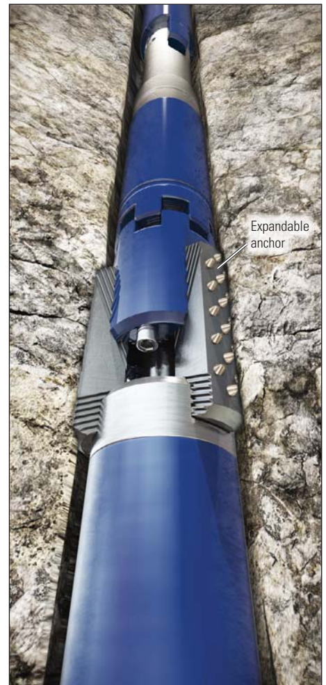
^ Hydraulic expandable anchor. This anchor's triaxial steel slips can expand to 150% of their original outside diameter to ensure a firm hold across a range of hole sizes.
