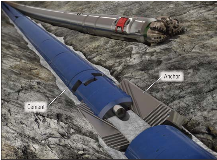
^ Sidetracking after pumping cement. With its anchor in place, the TrackMaster OH-C system permits drillers to sidetrack without having to wait for cement to cure.
