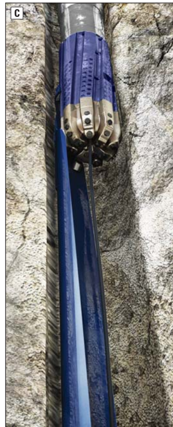
^ Bit and mill options. The bit or mill is attached to the top of the whipstock before it is run in the hole. On an openhole assembly, the bit is attached to the whipstock by shear pins. The openhole system can accommodate PDC (A), roller cone (B) or diamond-impregnated bits (C). Cased hole mills (D) are attached to the top of the whipstock by a break bolt. After the whipstock is oriented and the anchor is set, the bit or mill is separated from the whipstock by exerting upward or downward force to shear the attachment points.
