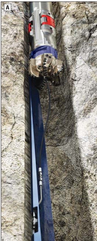
^ Bit and mill options. The bit or mill is attached to the top of the whipstock before it is run in the hole. On an openhole assembly, the bit is attached to the whipstock by shear pins. The openhole system can accommodate PDC (A), roller cone (B) or diamond-impregnated bits (C). Cased hole mills (D) are attached to the top of the whipstock by a break bolt. After the whipstock is oriented and the anchor is set, the bit or mill is separated from the whipstock by exerting upward or downward force to shear the attachment points.
