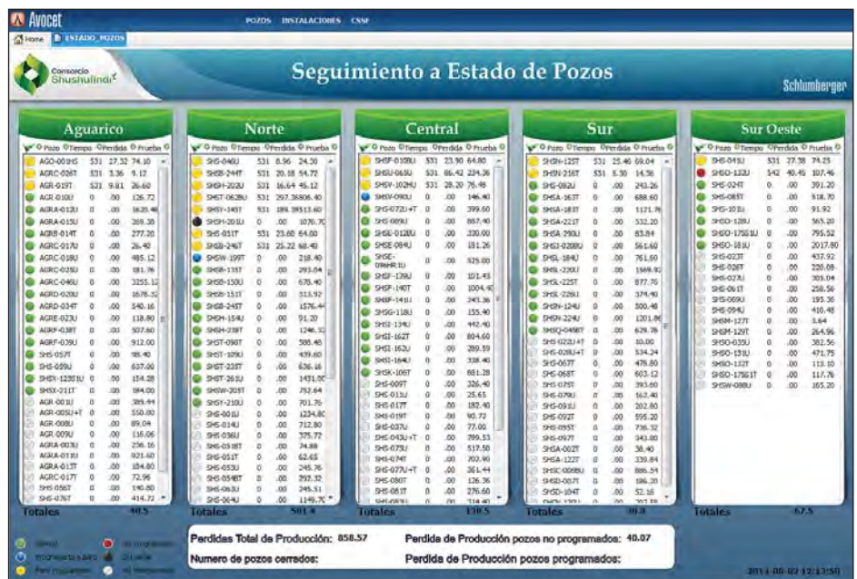
▲ Daily well monitoring status report. For each production area in the Shushufindi-Aguarico oil field—Aguarico, north, central, south and southwest—a panel contains four columns of the well status data, unscheduled downtime, lost production and latest well test flow rate. The circles on the left of each panel are color coded for the well status: normal (green), shutdown for well test (blue), scheduled shutdown (yellow), unscheduled shutdown (red), no signal from monitoring equipment (black) and not monitoring (white). At the bottom of each panel is the total unscheduled lost production for the area. The summary below the panels gives the cumulative production lost for the day, the number of shut-in wells and the production lost from unscheduled shutdowns and scheduled shutdowns.
