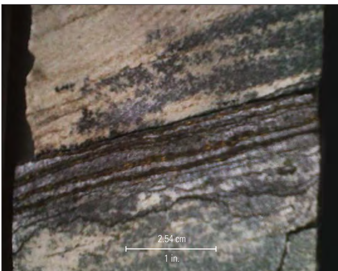
^ Cores from the Shushufindi field. Fine layers of coal and amber intercalate between clean siltstone mixed with shale (left). These dipping layers are preserved at the base of the sand bedsets and are typical of tidally dominated sediments. A photomicrograph (right) shows amber within coal. The preservation of amber is indicative of a quiet, low-energy sedimentary environment.
