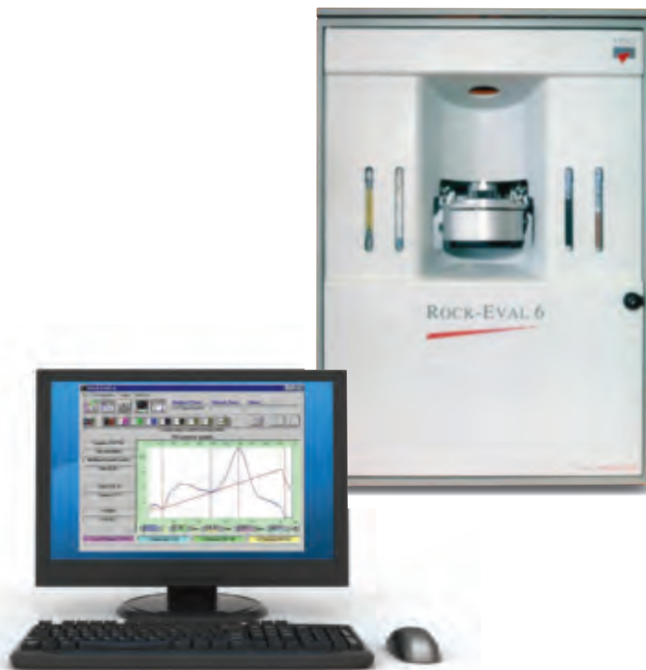
^ Pyrolyzer. This Rock-Eval 6 pyrolysis analyzer records gases evolved from the source rock during a programmed heating process. (Photograph courtesy of Vinci Technologies SA.)
