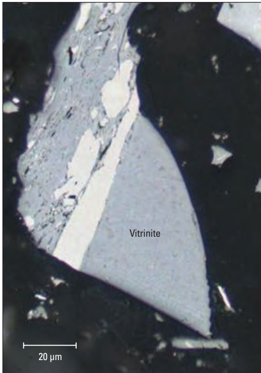
^ Vitrinite in bituminous coal. The amount of light reflected by vitrinite macerals is a key test for determining the thermal maturity of a rock. The intensity of light reflected from a sample is measured at hundreds of points along a microscopic sampling area, then a statistical analysis determines the amount of vitrinite in the sample and its thermal maturity. This photograph was taken in incident white light, with the sample in an oil immersion. [Photograph courtesy of the US Geological Survey Energy Resources Program: "2011 Photomicrograph Atlas," http://energy.usgs.gov/Coal/OrganicPetrology/PhotomicrographAtlas.aspx (accessed July 7, 2011).]
