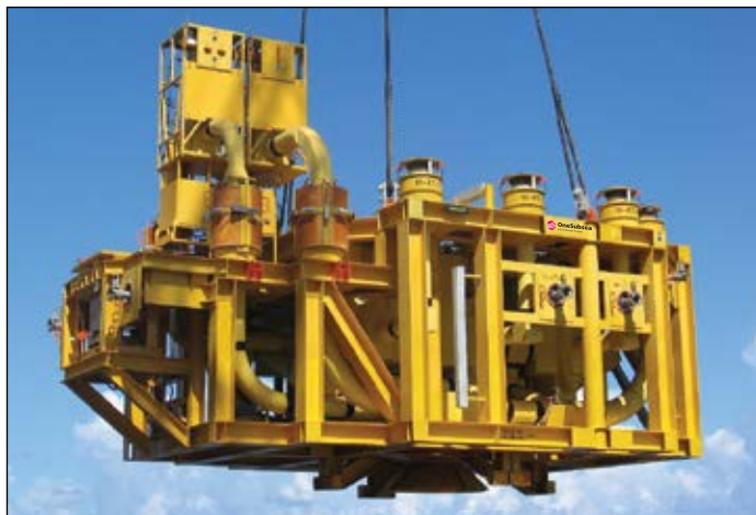
Figure 1. Subsea manifold. This manifold, hoisted in preparation for installation on the seafloor, will take produced fluids from several wells and route them to a flowline running to a production platform.
