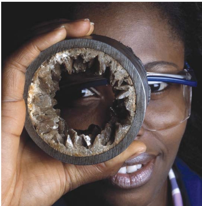
▲ Scale buildup in production tubing. Scale causes reduced flow rates and can, eventually, completely block production.
