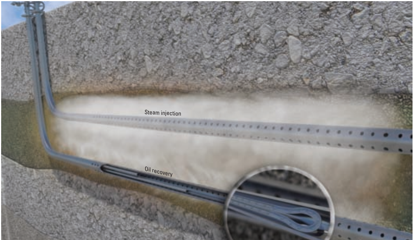
^ WellWatcher BriteBlue fiber installation in a heavy-oil well. Engineers pump the fiber through a conduit inside a coiled tubing string ( inset ) that is hung from the surface across the producing interval.
