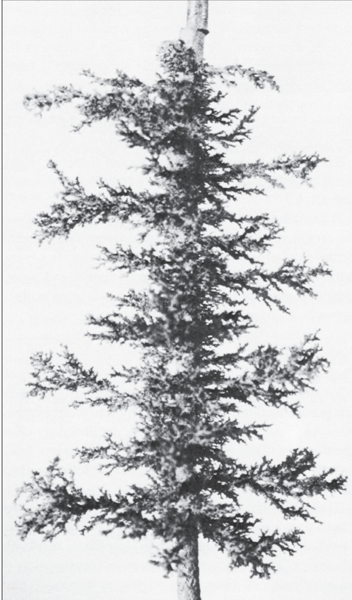
^ Wormholes formed during a laboratory-scale matrix acidizing treatment of a carbonate-formation sample. The length, direction and number of wormholes depend on the formation reactivity and the rate at which acid enters the formation. Once formed, the wormholes carry virtually all of the fluid flow during production.
