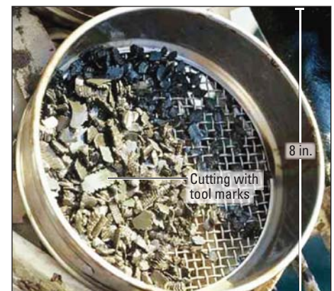
^ Cuttings from a PDC bit. Claystone in a mud logger's sieve shows tool marks, evidence of shearing action by a PDC bit.
