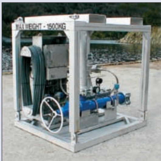
▲ Portable flowmeter. The PhaseTester multiphase flowmeter is housed in a modular framework (left). At 3,750 lbm [1,705 kg], the PhaseTester flowmeter is compact enough to be transported by a mid-sized truck (right).
