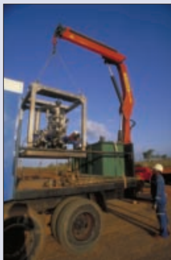
▲ Portable flowmeter. The PhaseTester multiphase flowmeter is housed in a modular framework (left). At 3,750 lbm [1,705 kg], the PhaseTester flowmeter is compact enough to be transported by a mid-sized truck (right).
