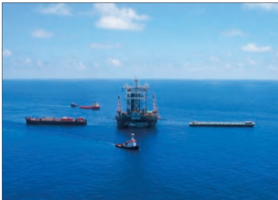
▲ Preparing to test. The Jack 2 well, originally drilled by the Discoverer Deep Seas drillship, was cased and suspended before moving in the Cajun Express semisubmersible rig for the extended well test. Barges were brought in beforehand to collect fluids produced by the test.
