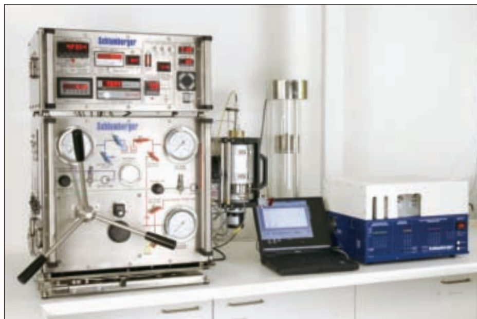
▲ Portable fluid analysis laboratory. The PVT Express mobile analysis service can provide information about the physical characteristics, composition and behavior of reservoir fluids. By bringing the laboratory to the wellsite, the operator can quickly obtain a detailed analysis of fluid composition, bubblepoint or dewpoint pressures, compressibility, viscosity and other important parameters.
